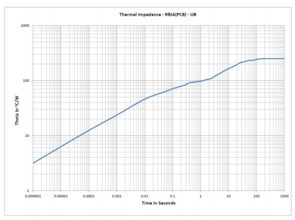
R0JA(PCB) = 250°C/W Thermal Impedance Note: Z0JX = 45°C/W maximum @10mS
