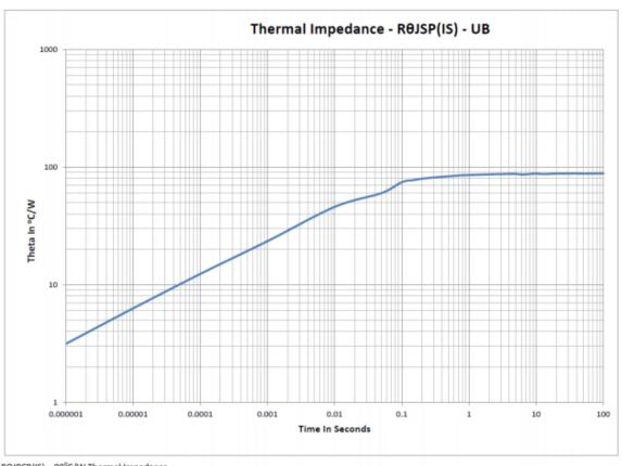
ROJPCB(IS) = 90°C/W Thermal Impedance Note: ZOJX = 45 °C/W maximum @10mS
