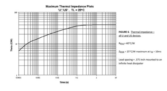
Maximum Thermal Impedance Plots Axial parts, TL = 25°C
