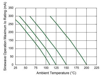
Sinewave Operation 50% Duty Cycle,  $R_{\rm BJA}$  (PCB) = 325°C/W. Maximum Finish-Alloy Temperature = 175°C
